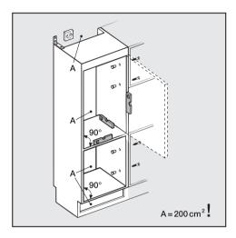
Before installing the appliance, the housing unit must be carefully aligned using a spirit level. The housing unit corners must be at right angles, as otherwise the appliance furniture door will not align correctly with the 4 corners of the unit. Align the furniture door with the hinges.
